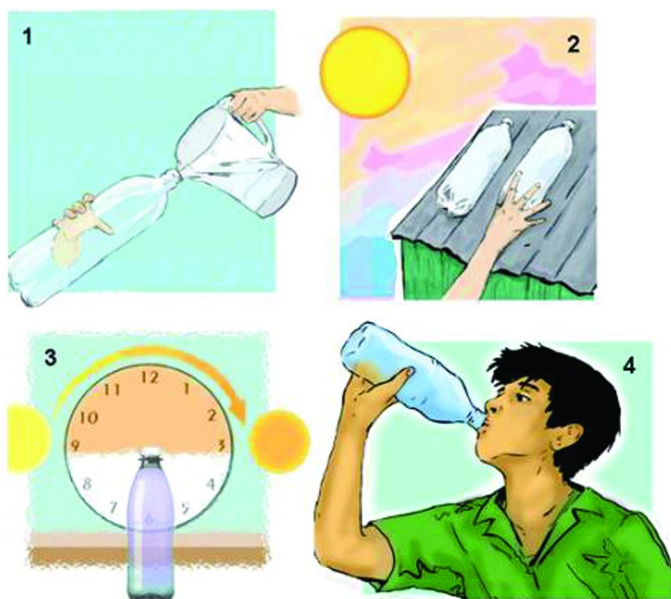
Figure 4. Simple protocol for the solar disinfection of water SODIS process. (courtesy of Dr. Kevin McGuigan, Royal College of Surgeons in Ireland, drawn by Maria Boyle).
